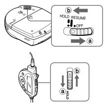
Release the HOLD switch before playback. → (a)
