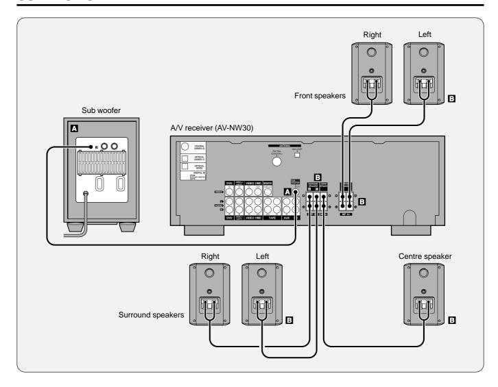
Before connecting the speakers, turn off the power of your stereo receiver and the sub woofer.
