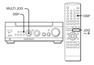
The DSP (Digital Signal Processor) surround circuits can recreate the effect of sounds reflected from walls or ceilings, to obtain the sound presence of real environments. The unit provides 10 DSP preset modes.
