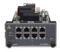
The DS1/E1 ATM IMA CMA is supported on the Alcatel-Lucent 7710 Service Router (SR-c4) and the 7710 SR-c12. The Alcatel-Lucent ATM IMA CMA is a hot-swappable, quarter-slot module with 8-port DS1/E1 over integrated RJ-48c interfaces, each capable of delivering wire-speed performance.
