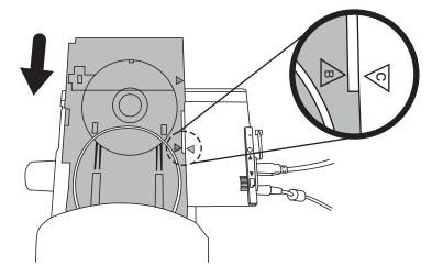
7. Click the "Tray Out" button so that the tray is pulled into the Autoloader
