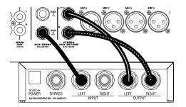
Alternatively, you may connect the output of the effect device to either of the STEREO LINE channels ([9-10 or 11-12].) This will allow you to control the effect with a large fader, send the effects to the Aux 1 output for monitoring, and use EQ on the effect.
