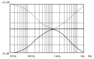
$oldsymbol{igsi}$  The normal position for the EQ controls is "12 o'clock" or straight up. A "click" or detent will be felt at this position. At this position, the EQ does not affect the frequency response of the channel--it is "flat".
