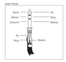
(the ring of a TRS plug). A special Y-cable consisting of a TRS 1/4" plug on one end and two mono 1/4" plugs on the other end is required.
