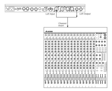
**Stereo.** In the case where a stereo instrument, such as a keyboard or sampler, is connected to two separate channels of a mixing console, you will need two 1/4" TRS cables, one for each channel. The connection is made in a similar fashion as described above.
