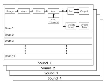
Here is a block diagram of a sound in Drum Mode.
