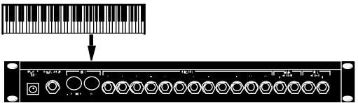
The [MIDI OUT/THRU] connector sends MIDI data from the DM5's keyboard to other MIDI devices, but can also send *System Exclusive* data (see the MIDI supplement in Appendix B) to a storage device for later recall. You can also convert the signals generated by the external triggers into MIDI signals to send out to other MIDI devices (such as a sequencer).
