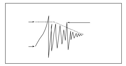
This chart simulates the waveform of a snare drum hit. The first big point in the signal is the actual hit, the rest of the waveform is all decay. Since the Decay time threshold is adjusted too low, the Decay level curves off too soon allowing a second point, during the signal's decay, to exceed the threshold. Once this happens the DM5 will trigger the sound.
