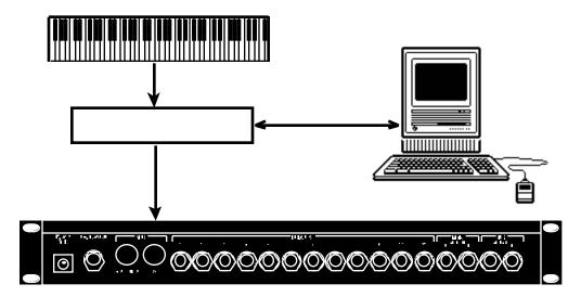
This allows you to record into the sequencer by playing on your MIDI keyboard / controller, and have the sequencer play back what you have recorded on the DM5.
