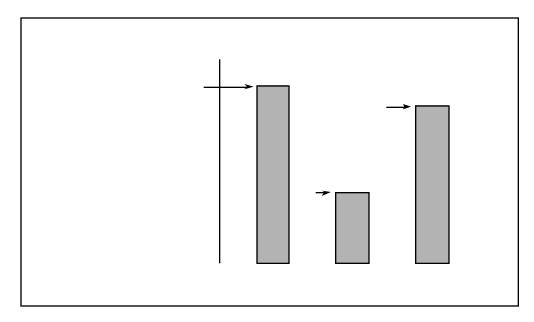
This chart represents three signals which are "seen" by the DM5. Signal 1 is a legitimate hit from the snare pad. Signal 2 is the Tom 1 pad, but it is not a hit. It is the pad being triggered by stand vibrations from the first snare hit. Signal 3 is a second "real" hit from the snare pad.
