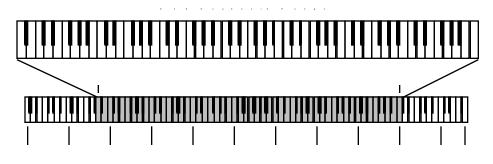
By setting the lower limit above the high limit, you can create a "hole in the middle"
