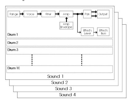
When Drum Mode is enabled, the sound will have fewer parameters for editing. Consequently, not all Function buttons will respond when pressed as when Drum Mode is turned off. Specifically, the LFOs and all Envelopes (with the exception of the Amp Envelope) are unavailable. In addition, the parameters in most other functions will differ.
