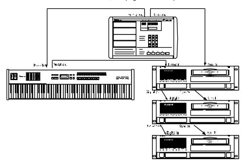
*Tip:* With this type of connection, the ADAT tracks will remain in tune with the QS even when the BRC's pitch value is adjusted.
