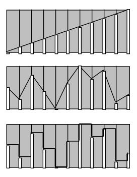
The Tracking Generator can be used to turn a variable control, such as the Mod Wheel or velocity, into a switch by setting all of the points to 0 except for point 10. Only near the maximum input will anything other than 0 come out of the Tracking generator. You can patch the Mod Wheel somewhere else in addition to the Tracking Generator, giving you gradual control of one function with the full range of the Mod Wheel, while switching on a second function only at the top of the wheel.
