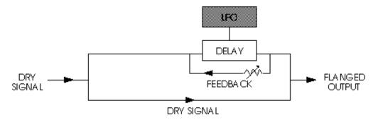
Many variables are available, from varying the speed and depth of the LFO to feeding back part of the signal to make the effect stronger. The Flanger's feedback can be either "Normal" or "Inverted". Use the "Inverted" setting for a more dramatic flange effect.
