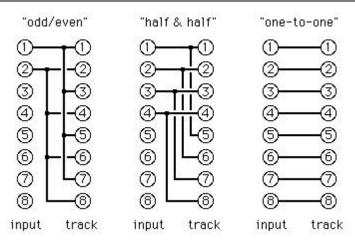
**Note:** The above illustrations assume that the source tracks of the M20 are set to receive digital input (as shown by a "D" under the meter for each track).
