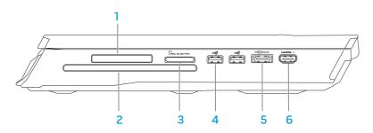
ExpressCard slot — Provides support for additional memory, wired and wireless communications, multimedia, and security features. The slot supports 54 mm Express cards.
