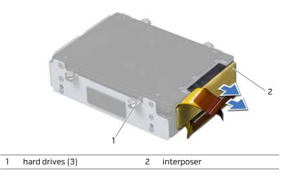
Remove the screws that secure the hard drive(s) and slide the hard drive(s) out of 5 the hard-drive bracket.
