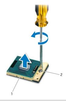
1 ZIF socket 2 ZIF-socket cam screw
