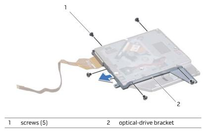
Remove the interposer from the optical drive.
