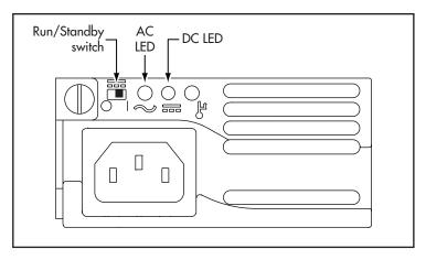
Note that when the Run/Standby switch is set to the Standby position (0), the AC LED lights and the fan spins, but the DC LED does not light and the PSU **does not** deliver power to the device.
