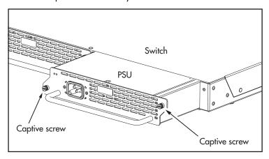
If a unit is already in the bay, slide it out slowly and carefully. Support the unit from underneath as you remove it to prevent it from falling.
