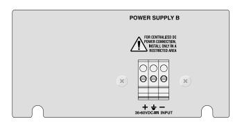
2. With a 14-gauge wire-stripping tool, strip the three wires in the tray cable coming from the DC input power source to 8 mm  $\pm$  1 mm (0.31 in  $\pm$  0.039 in).
