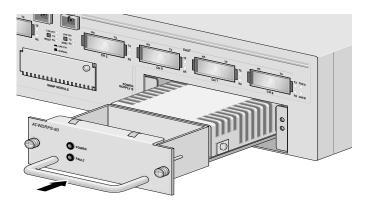
4. Secure the AT-WDRPS-80 unit to the AT-WD1008 chassis by tightening the two
