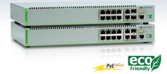
The AT-8100L/8POE-E is a Layer 2 to 4 small form factor Ethernet switch designed for harsh environments. Unlike traditional DC powered industrial networking equipment, the -E Series products are optimized for the middle ground requirement that needs classic AC powered enterprise switches, that ensure high reliability and are tested to withstand higher temperatures, shock and vibration.
