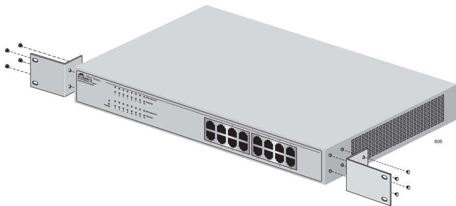
Figure 10. Attaching Rackmounting Brackets
