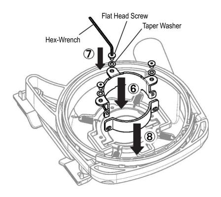
8. Tighten the Screws (DO NOT forget to insert Spring Washers)
