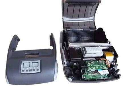
3. Use a tool to remove the shaft. Remove/Replace the media cover. (including the platen roller ass'y)
