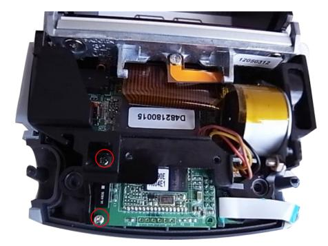
3. Disconnect the connector on the board.
