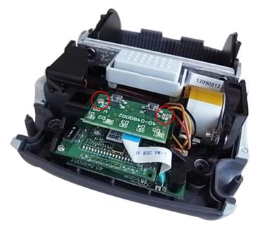
3. Loosen the connector lock then disconnect the flat cable from the keys control board. Remove/Replace the keys control board.
