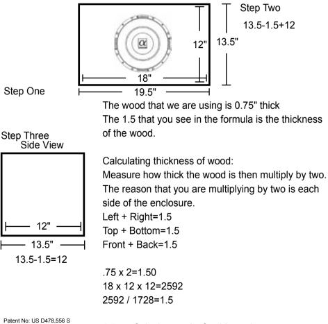
Calculating speaker enclosure volume is a five step procedure. (Make sure you do not forget to subtract the thickness of the wood and port displacement that you used.)
