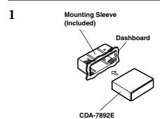
Slide the mounting sleeve into the dashboard.
