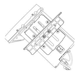
4 Note that the vehicle-side brackets allow for easy radio position adjustment during installation.
