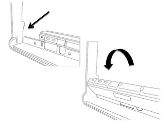
7 Plug in the key connection harness with the "external key unit" label to the key unit and the 3.5mm "MIC IN" pig tail to the head unit. Note the pigtail connection for the included Bluetooth microphone.
