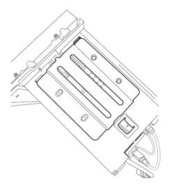
2 Assemble the radio and vehicle side brackets using the supplied bracket screws and washers. Tighten these bolts just enough so that the brackets can be repositioned if necessary. **3** Bolt the assembled brackets to the radio chassis using the supplied 8mm screws.
