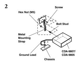
Reinforce the head unit with the metal mounting strap (not supplied). Secure the ground lead of the unit to a clean metal spot using a screw (\*) already attached to the vehicle's chassis.
