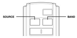
Press the BAND button on the CDA-9807/CDA-9805 or the RUE-4187 to activate the CD Changer Selection mode. 3 The CD Changer Selection mode remains active for 8 seconds after step 2 is performed. Press the BAND/TEL. button until the desired CD Changer indicator appears on the display.
