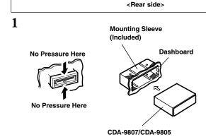
Remove the Detachable Front Panel (refer to page 5). Slide mounting sleeve from main unit. (see "Removal" on this page).
