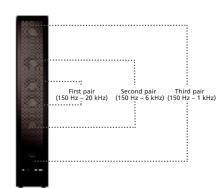
Low pass filtering actively directs specified frequencies of sound to a different pair of micro drivers. This process, combined with the critical distance between each micro driver, creates the focused coverage pattern in front of the flat panel display.
