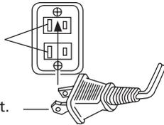
Insert the wide blade into the ground side slot.
