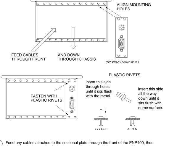
1 down through the opening in the bottom of the chassis. Make sure the cables exit the chassis on the same side as the plate. They should NOT cross over the center of the unit.
