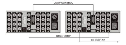
In this configuration the loop control pin 6 on the 9 pin D connector is connected to the same pin on all switchers.
