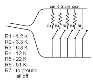
In some cases it may be preferable to use a seven conductor wire to control the switcher with contact closures. The **RC5204CC** adapter is available to accommodate this need. The pin outs for this adapter are as follows:
