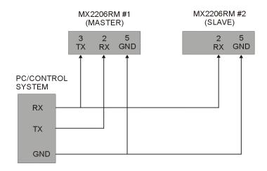
If you want to make 11 by 1 switcher using two 6 by 1 switchers, the following commands need to be used to control these switchers:
