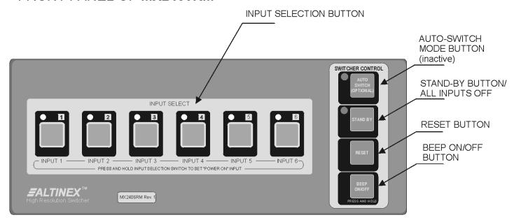
The front panel of the **MX2406RM** provides access to essentially all of the switcher's capabilities. In addition to standard switching functions, the unit has control and switching functions that could be very useful in a variety of special applications.
