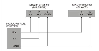
If you want to make 11 by 1 switcher using two 6 by 1 switchers, the following commands need to be used to control these switchers:
