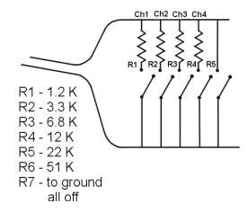
In some cases it may be preferable to use a seven conductor wire to control the switcher with contact closures. The **RC5204CC** adapter is available to
