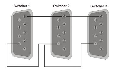
More specifically, the output of one switcher is connected to INPUT 6 of the next switcher. Once loop control is enabled these switchers will automatically switch video signals to the output of the second switcher through INPUT 6. Keep in mind that you are always going to have one less input than the total number of inputs available on all switchers. The figure above is for an 11-in 1-out switcher.
