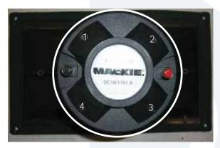
The horn assembly is shown above with the high frequency driver circled. Four screws need to be removed from the driver using the 3mm allen wrench.
