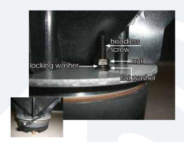
Four nuts and eight washers may be removed from the definition removed from the driver using the 8mm open end wrench. Turn counterclockwise to loosen and remove, clockwise to tighten. The other three are located around the horn assembly. Lift the horn up as the nuts are loosened. It cannot be removed otherwise. Notice that the flat washer is on the bottom, followed by the locking washer, and finally the nut.
