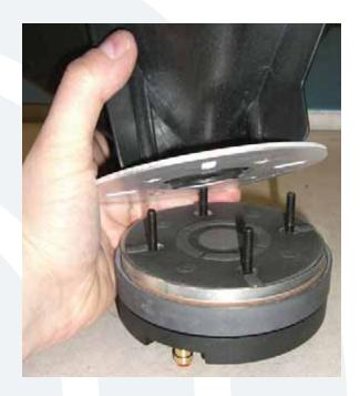
The horn assembly should easily lift right off of the high frequency driver.
