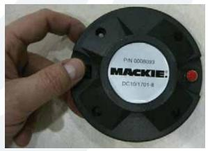
This is what the plate adapter and diaphragm look like after they have been removed from the horn assembly. The diaphragm is separated from the plate adapter simply by pushing down on the terminals.
