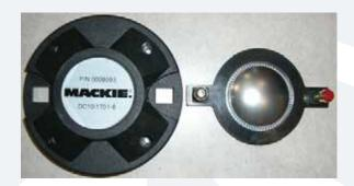
7 This is what the plate adapter (left) and diaphragm (right) both look like. Place the new diaphragm (part # coming soon) where the old one was. Follow the same steps as above, but backwards 6 to 1. Power up the S215 and the new diaphragm should now be pumping out those highs again. Sweet, you just replaced a diaphragm!
