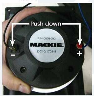
The positive (solid blue) and negative (solid black) cables are still attached to the high frequency driver terminals. Remove the cables from their terminals simply by pushing down on the terminal and pulling out the cable.
