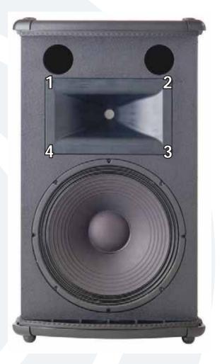
Four screws and flat washers need to be removed from the horn assembly using the 5mm allen wrench.
