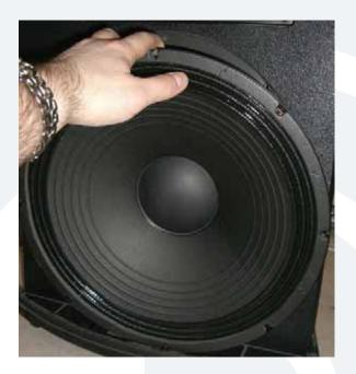
Carefully begin to remove the woofer. This woofer has a tendency to want to pop out, so please be sure to hold the woofer in place with your free hand while removing the screws with the other hand.
