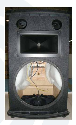
7 The picture above shows what the S215 looks like with the grill and woofer removed. Place the new woofer (part #0010658) where the old one was. Follow the same steps as above, but backwards 6 to 1. Power up the S215 and the new woofer should now be pumping out glorious lows. Awesome, you just replaced a 15" woofer!
