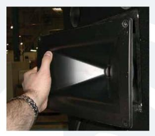
Carefully begin to remove the entire horn assembly (with the high frequency driver still attached). A flat head screwdriver may aid in loosening the horn assembly by prying between it and the cabinet. Hold the horn assembly in place with one hand while prying around the edge with your free hand.
