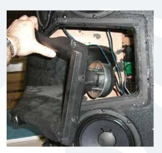
Carefully begin to remove the entire horn assembly (with the high frequency driver still attached). Caution: The horn weighs about 8
