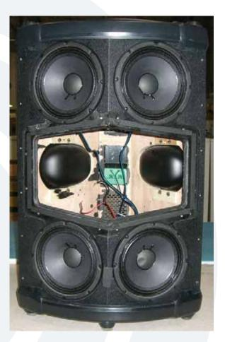
5 This is what it looks like with the grill and horn assembly removed. See the next page for further instructions and additional pictures on how to remove and replace the high frequency driver.
