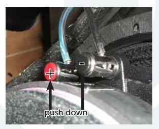
The positive (blue and black) and negative (solid black) cables are still attached to the woofer terminals. Remove the cables from their terminals simply by pushing down on the terminal and pulling out the cable.
