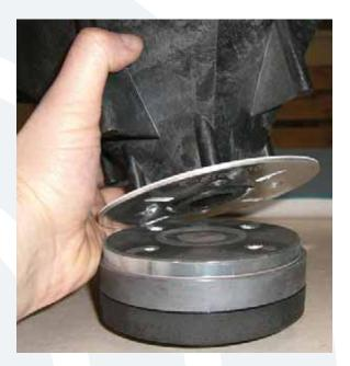
The horn assembly should easily lift right off of the high frequency driver. Place the new high frequency driver (part #0008093) where the old one was. Follow the same steps as above, but backwards 8 to 1. Power up the S408 and the new driver should now be pumping out those highs again. Fantastic, you just replaced a high frequency driver!
