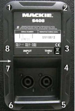
Eight screws need to be removed from the input assembly (located on the rear of the cabinet) using the phillips head screwdriver. Once the screws are removed, the input assembly may be loosened by prying a flat head screwdriver in between it and the cabinet. Keep the eight screws in a safe place.
