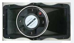
The horn assembly is shown above with the high frequency driver circled. Four screws need to be removed from the driver using the 3mm allen wrench.
