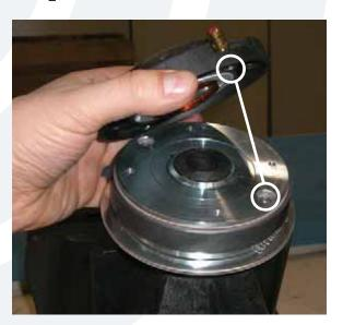
The diaphragm and plate adapter are easily removed from the horn assembly. Notice the terminal locations in relation to the indents of the high frequency driver (circled above).
