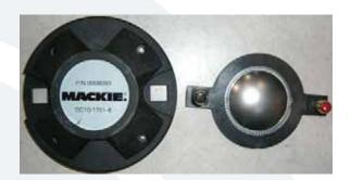
This is what the plate adapter (left) and diaphragm (right) both look like. Place the new diaphragm (part # coming soon) where the old one was. Follow the same steps as above, but backwards 6 to 1. Power up the \$408 and the new diaphragm should now be pumping out those highs again. Sweet, you just replaced a diaphragm!
