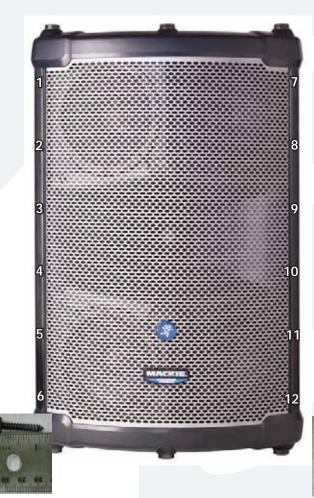
Six screws need to be removed from each side of the front of the grill (twelve screws total) using the phillips head screwdriver. This grill has a tendency to want to "pop" off, so please be sure to hold it in place with one hand or arm while removing the screws with your free hand. In addition to the grill, the screws also hold the decorative trim. The trim should be removed, too. Keep the twelve screws in a safe place.
