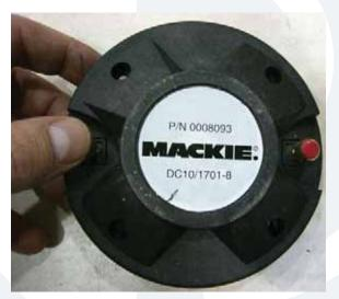
This is what the plate adapter and  $(\mathbf{0})$ diaphragm look like after they have been removed from the horn assembly. The diaphragm is separated from the plate adapter simply by pushing down on the terminals.
