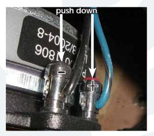
The positive (blue and black) and negative (solid black) cables are still attached to the woofer terminals. Remove the cables from their terminals simply by pushing down on the terminal and pulling out the cable.
