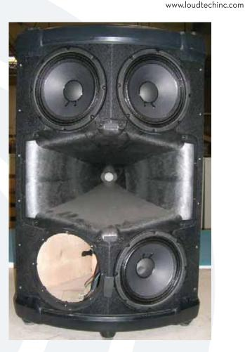
The picture above shows what the S408 looks like with the grill and bottom left woofer removed. Place the new woofer (part #0011806) where the old one was. Follow the same steps as above, but backwards 4 to 1. Power up the S408 and the new woofer should now be pumping out glorious lows. Awesome, you just replaced an 8" woofer!
