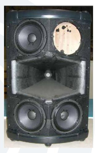
The picture above shows what the S408 looks like with the grill and top right woofer removed. Place the new woofer (part #0011806) where the old one was. Follow the same steps as above, but backwards 4 to 1. Power up the S408 and the new woofer should now be pumping out glorious lows. Awesome, you just replaced an 8" woofer!
