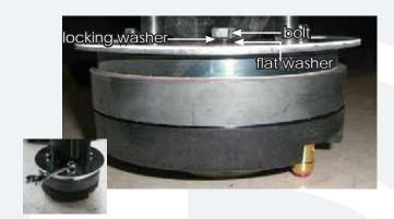
Four bolts and eight washers may be removed from the driver using the 8mm combination wrench. Turn counterclockwise to loosen and remove, clockwise to tighten. The other three are located around the horn assembly. Notice that the flat washer is on the bottom, followed by the locking washer, and finally the bolt.
