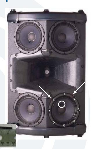
Six screws need to be removed from each side of the front of the grill (twelve screws total) using the phillips head screwdriver. This grill has a tendency to want to "pop" off, so please be sure to hold it in place with one hand or arm while removing the screws with your free hand. In addition to the grill, the screws also hold the decorative trim. The trim should be removed, too. Keep the twelve screws in a safe place.
