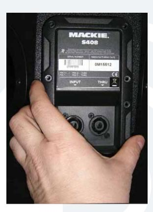
2 Once loosened, the input assembly may be easily removed from the cabinet. Do not completely take the input assembly off yet, as two cables need to be removed first.
