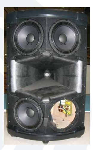
The picture above shows what the \$408 5 looks like with the grill and bottom right woofer removed. Place the new woofer (part #0011806) where the old one was. Follow the same steps as above, but backwards 4 to 1. Power up the \$408 and the new woofer should now be pumping out glorious lows. Awesome, you just replaced an 8" woofer!
