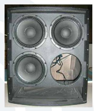
The picture above shows what the S410s looks like with the grill and bottom right woofer removed. Place the new woofer (part #0011737) where the old one was. Follow the same steps as above, but backwards 4 to 1. Power up the S410s and the new woofer should now be pumping out glorious lows. Awesome, you just replaced a 10" woofer!
