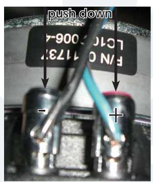
The positive (blue and black) and negative (solid black) cables are still attached to the woofer terminals. Remove the cables from their terminals simply by pushing down on the terminal and pulling out the cable.
