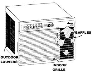
may collect and block unit air flow. If air flow is obstructed or deflected back into unit, the compressor may cycle on and off rapidly, causing early compressor failure.
