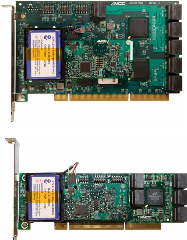
Figure 30. BBU installed on controllers
