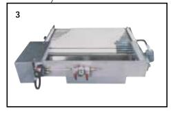
Special diverter with aligner and pneumatically operated drop gate. Aluminum and stainless steel construction. This unit transports and facilitates smooth transfer of dough pieces onto desired position of freezer belt. Above shown with:
