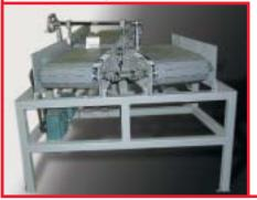
The switch consist in three conveyors mounted on a single rigid frame. One conveyor is pivoting around a vertical axis (from one side to the other), the two receiving conveyors are fixed.
