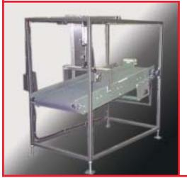
Our Vertical Selector Switch is used to switch Pans, Lids, Trays, Baskets or Products from one Conveyor Line into two or three superposed (same vertical plane) receiving lines. This type of switch is generally used when the selection of the receiving conveyor lines is made prior to the start-up of the production, generally the switching is not possible while running.
