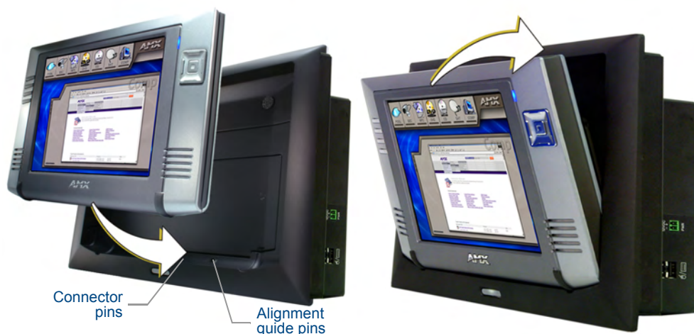
FIG. 16 Installing an MVP onto an MVP-WDS
