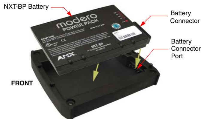
FIG. 25 Battery installation
