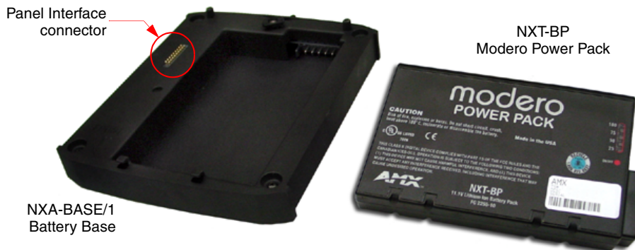
FIG. 23 NXA-BASE/1 Kit (consists of one BASE/1 and a single NXT-BP)
