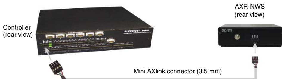
FIG. 7 AXR-NWS connection to a Controller
