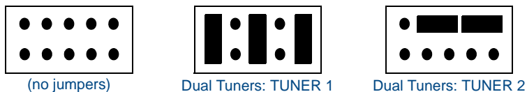
FIG. 61 Tuner Module Jumper Configuration (Red Interface Boards)
