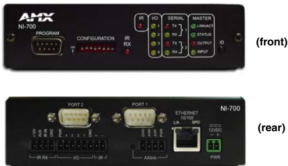
FIG. 1 NI-700 NetLinx Integrated Controller (front and rear views)
