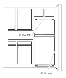
To ensure proper ventilation for your refrigerator, allow for a  $\frac{1}{2}$ " (1.3 cm) space on each side. Allow 3" (7.5 cm) of space between overhead cabinets and refrigerator top. Allow at least 1" (2.5 cm) between back of cabinet and the wall. If your refrigerator has an ice maker, make sure you leave some extra space at the back for the water line connections.
