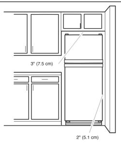
To ensure proper ventilation for your refrigerator, allow for a 1/2" (1.3 cm) space on each side. Allow 3" (7.5 cm) of space between overhead cabinets and refrigerator top. Allow at least 1" (2.5 cm) between back of cabinet and the wall. If your refrigerator has an ice maker, make sure you leave some extra space at the back for the water line connections.
