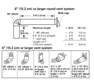
Calculating Vent System Length To calculate the length of the system you need, add the equivalent feet (meters) for each vent piece used in the system.
