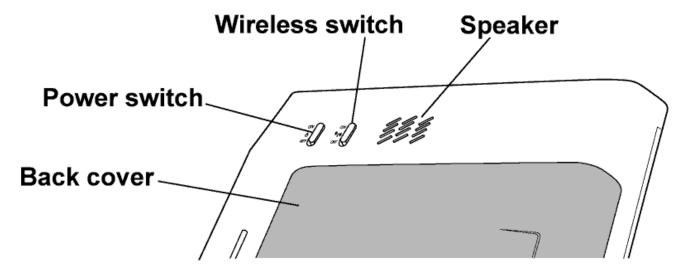
**Power switch** — turns your Kindle on or off. However, instead of turning your Kindle off when you are done reading, you can just hold down the ALT key and then press and release the Text key to put your Kindle to sleep. This will extend your battery life and locks all of the other keys and buttons on Kindle so you don't accidentally change the place in your reading.
