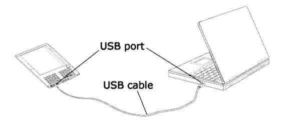
When you are connected to your PC, the Kindle screen will change to show the USB drive mode screen. Your Whispernet service is temporarily shut off and you will not receive any of your subscriptions while in this mode. Also, your Kindle is not usable as a reading device while you are
