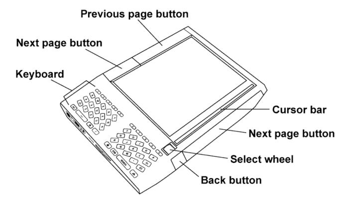
**Cursor bar** — contains the cursor, which is a silver rectangle that allows you to select a particular line on the display. You move the cursor up and down the bar using the select wheel. When the cursor is lined up with what you want to select, press down and release the select wheel to make your selection.
