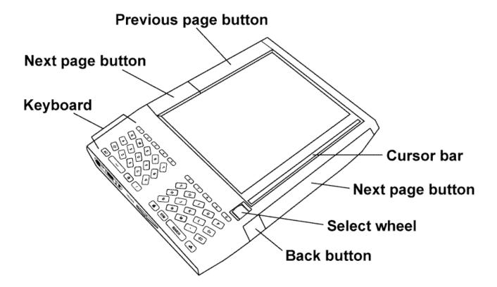
To choose a particular item such as a menu choice or a line of text in what you are reading, roll the select wheel to move the silver cursor up and down the cursor bar and then press and release the select wheel to make your choice. Try rolling the select wheel now.
