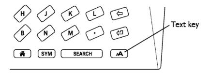
If you would like to try it now, simply press the text key , roll the select wheel to move the cursor next to the size you prefer from the menu, and press the select wheel. The text is now shown in the new size. Repeat the same steps to change the text size back or to change it to a different size that is most comfortable for you to read.
