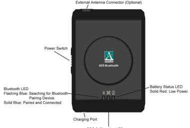
GPS & Charging LED Flashing Green: Searching for GPS Satelites. Solid Green: GPS Satelites position fixed. Flashing Red: Charging. If your GPS receiver device is turn off, the red charging LED will flash while charging and turn off when fully charged.
