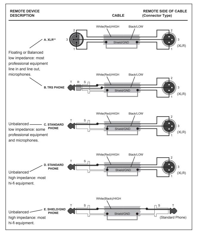
Connector and cable configurations are recommended for use with the M 4 bus series. These cables are based on the use of auxillary equipment that is isolated from the AC power mains.
