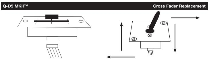
The crossfader is "Hot Swappable" which means it may be replaced at any time, even when power is applied. Only replace with American Audio Part OF-1. Replacing with any other model fader may seriously damage your mixer.
