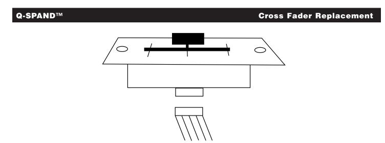
The crossfader is "Hot Swappable" which means it may be replaced at any time, even when power is applied. Only replace with American Audio Part Feather Fader Plus. Replacing with any other model fader may seriously damage your mixer.
