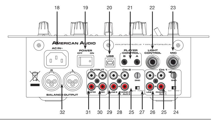
**18. AC CONNECTION -** This connector is used to supply main power to the unit via the included detachable power cord. Use only the supplied, polarized AC power cord. This cord is designed to fit in one direction only. Do not attempt to force a cord in if it does not fit, be sure the cord is being inserted properly
