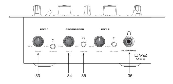
**33. CHANNEL FADER CURVE ADJUSTMENT -** This rotary knob is used to change the way the channel fader will operate. Each of the two channels has a "Curve" adjustment. The curve on the faders adjust from long or short or any variation of the two. The shorter the curve adjustment the sooner full volume will be reached.
